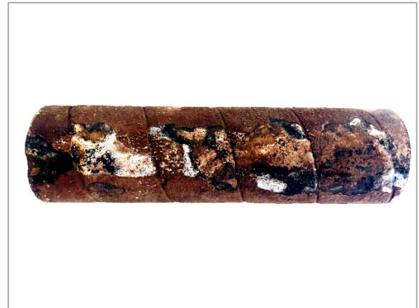
Plate 1: Boiler firetube with widespread corrosion.
